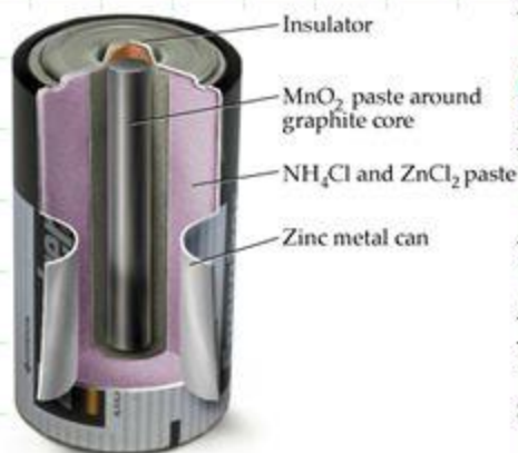
Cross-section of a dry cell
