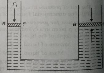
If a downward force  $F_1$  is applied. On the piston A, then the pressure exerted on the liquid is
