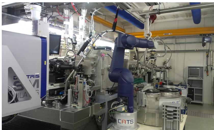
An experimental station used for X-ray crystallography at a synchrotron beamline. A protein crystal mounted in the beamline, where it is cooled by a stream of cold nitrogen gas, is shot with X-rays and its diffraction pattern collected on an X-ray detector. PSI SLS, Villigen, CH
