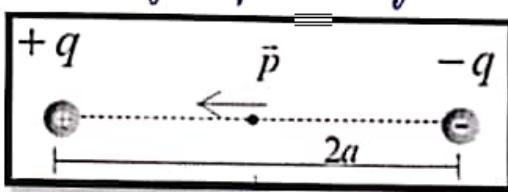
$$\text{Dipole moment } \vec{P} = q \vec{d} \quad [d = 2a \text{ here}]$$
