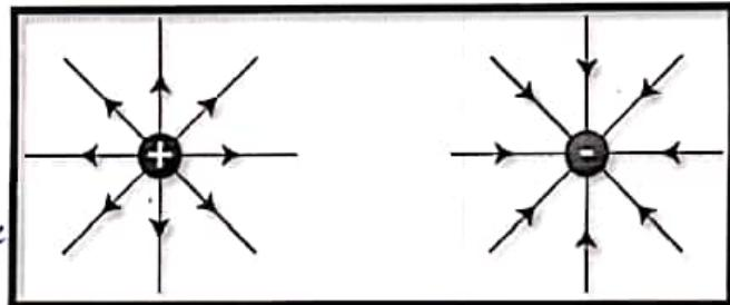
Lines of force are drawn in such a way that the tangent to a line of force gives the direction of resultant field there.
