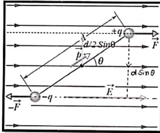
\*\* Work done in rotating a dipole in Electric field.
