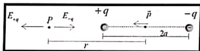
Q. Let us consider a point  $P$  at a distance  $r$  from the centre of the dipole. If  $E_q$  be the electric field at the point  $P$  due to the charge  $+q$  then  $|E_{+q}| = \frac{1}{4\pi\epsilon_0} \frac{q}{(r-a)^2}$  ... ①
